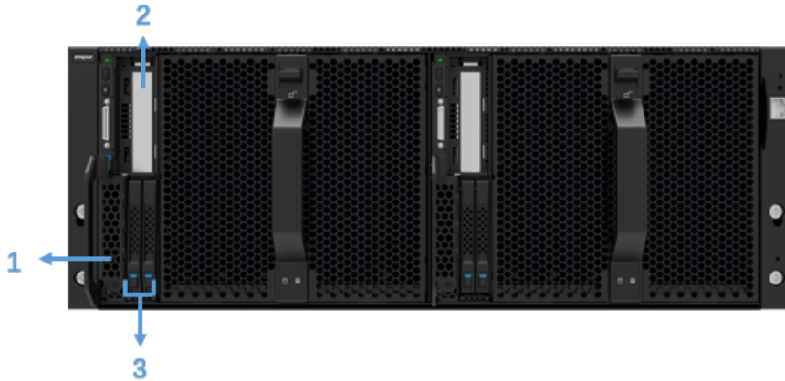
Figure 5-8 NS5486M6 2SSD 1LP Front View
